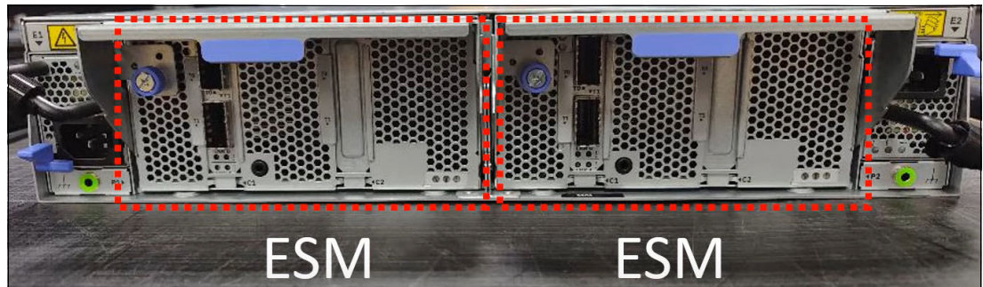
Figure 2-35 Back view of the NED24 Expansion Drawer
