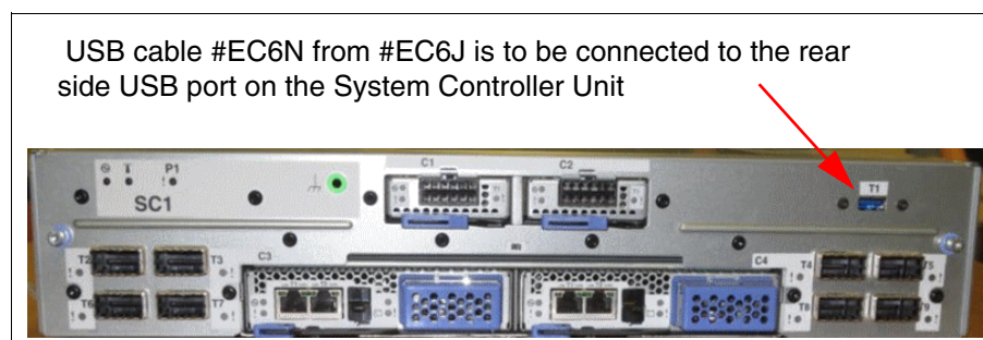
Figure 2-23 Rear view of the SCU showing the USB port for connection
