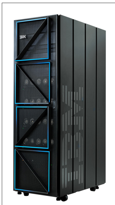
Figure 1-1 Power E1080 4-node server mounted in an S42 rack with a #ECRT door
